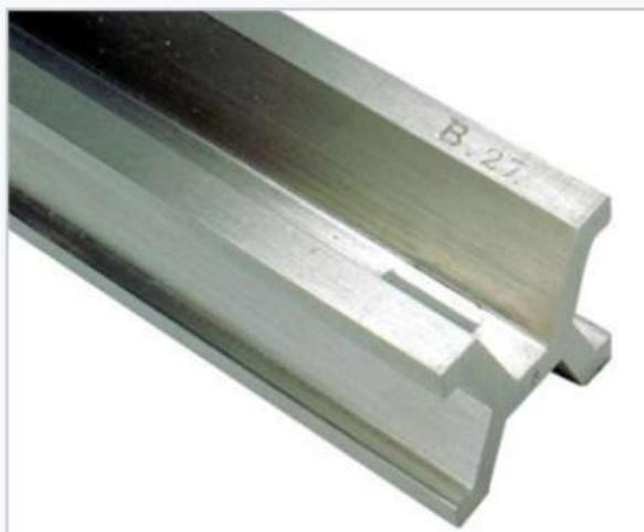
Closeup of National Prototype Metre Bar No. 27, made in 1889 by the International Bureau of Weights and Measures (BIPM) and given to the United States, which served as the standard for defining all units of length in the US from 1893 to 1960
