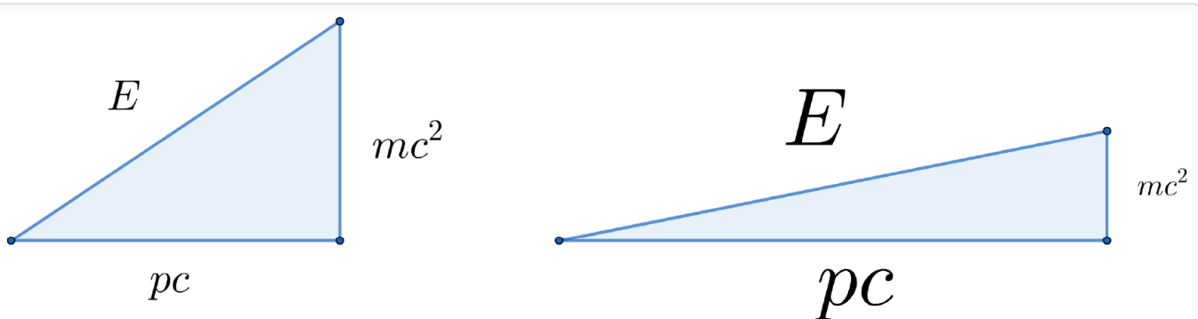
Figure 5. A triangle with a tiny vertical side Approaching the behaviour of light for massive objects by squeezing the hypotenuse ( E ) towards the adjacent ( pc ). Comparing the right triangle with figure 4, we see that it approaches the same shape and hence it
